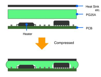
PG25A is the lowest modulus type of Putty Type available. Ideally suited for applications requiring low compression force on the component. It offers the high performance that very easily conforms in and around protrusions and depressions on components to make complete, reliable physical contact.
