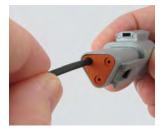
**Step 3:** Push contact straight into connector grommet until a click is felt. A slight tug will confirm that it is properly locked in place.
