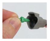
**Step 4:**Once all contacts are in place, insert green wedge. The green wedge will snap into place.
