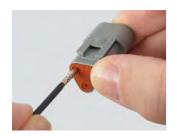
**Step 3:** Hold the rear seal in place, as removing the contact will displace the seal.
