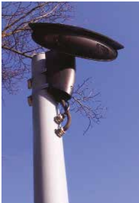
SafeWalk has been designed to detect stationary pedestrians, adjacent to the pole on which it is mounted.
