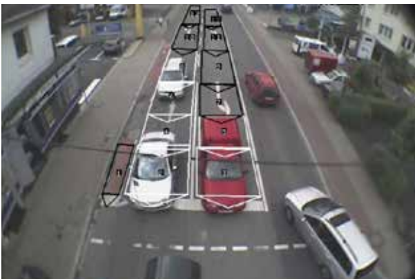
Traditional video cameras as well as thermal cameras can be combined with FLIR's traffic video analytics.
