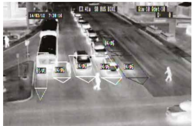
Traditional video cameras as well as thermal cameras can be combined with FLIR's traffic video analytics.
