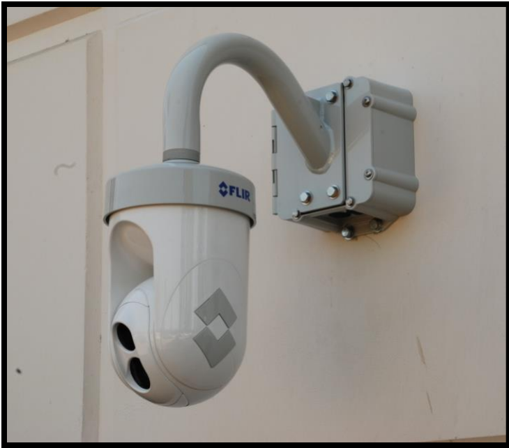
Concealed connections via rear panel
