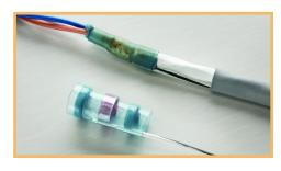
On many STS parts a special thermochromic coating on the solder preform changes color when it reaches the optimum temperature. This makes it easy for the operator to know when the proper amount of heat has been applied. This feature, plus the transparency of the sleeve make inspection simple. In one glance, it is possible to verify that the solder has melted, flowed, and is evenly distributed. Many STS products have a permanent identification number for easy recognition.
